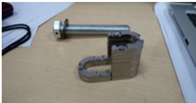
The two position stopper was made and installed
